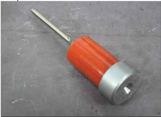
Each guide has a depression machined into the bottom face that fits snugly over the rivet, perfectly centering the drill bit on the head.
